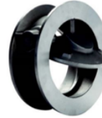
RM Check Valve Wafer type Stainless steel Metal seated DN40- DN900 PN10 -Pn40 Options: With counter lever and Weight of Spring
